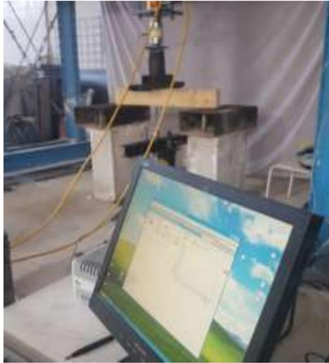
Figure 2. Device for flexural tests of beams
